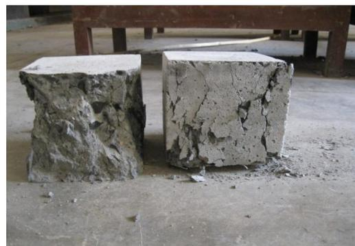
Photograph 2 Tested specimens of normal and PFRC
