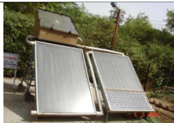
**Figure 6: Photograph of hybrid (PVT) Active solar still.**
